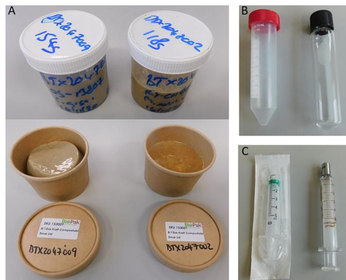
**Fig 2. Transition from A) 200 mL plastic pots to compostable paperboard pots for storage of shellfish samples, B) transition from 50 mL plastic to glass centrifuge tubes and C) transition from 5 mL plastic to glass syringes.**
