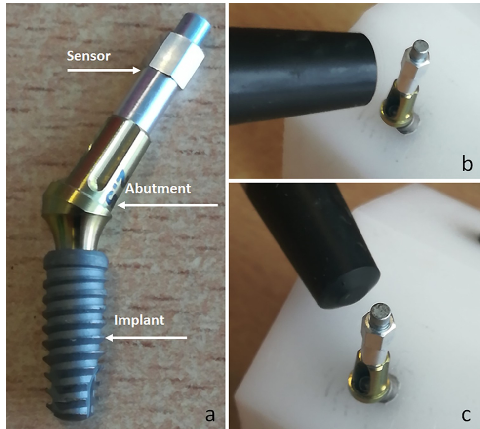
Fig 5. Representative image of the IA set, and the magnetic sensor installed (a). ASQ measurement in the frontal direction (b) and in lateral direction (c).
